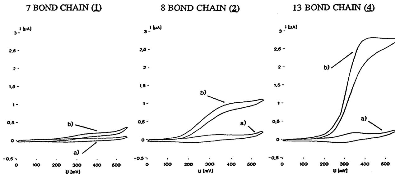
**Figure 3.** Effect of the chain length connecting peripherally bound ferrocene to glucose oxidase on the electrocatalytic glucose oxidation current. Curves a represent oxidation currents in the absence of glucose; curves b represent currents at 40 mM glucose. All solutions contain 2 mg mL<sup>-1</sup> of one of the modified enzymes, 0.1 M phosphate buffer (pH 7.2), and 200 units/mL<sup>-1</sup> catalase; 3-mm-diameter glassy carbon disks; all potentials vs SCE; scan rate 10 mV s<sup>-1</sup>.
